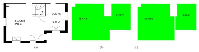
Figure 2: Room Spliting: Room part from original floor plan image(a) Room detection and labeling (b) Room Spliting using labeling results(c)
