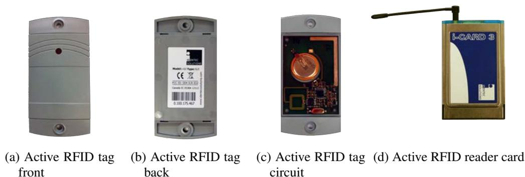
**Figure 4.24:** Active RFID tag by Identec Solutions as used in the LORIOT system. Each tag has a unique ID number that is also printed on the back of the housing (b). The tags are powered by coin cell batteries and the circuit contains an LED that can be used to indicate activity of each tag (c).
