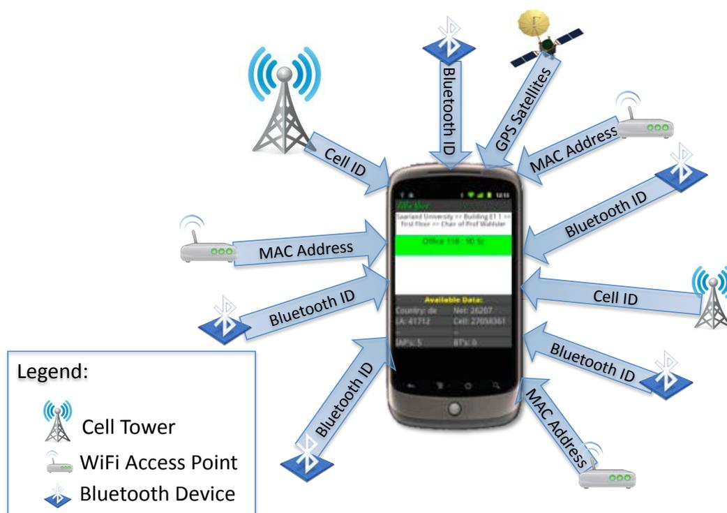
**Figure 4.13:** Sensors and senders of UBISPOT: GSM/UMTS cells, WiFi access points and Bluetooth devices act as senders. For outdoor positioning, GPS is used in addition.
