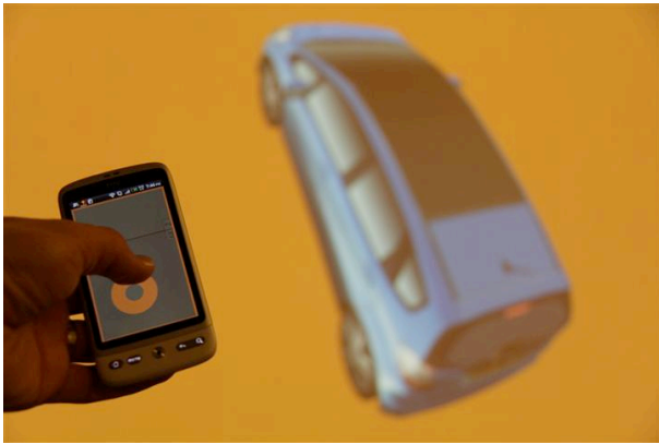
Figure 1: UNUC used to manipulate an object in 3D space: the object's orientation is controlled by the phone's orientation obtained from the phone's sensors.
