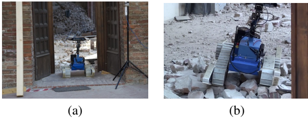
Fig. 1. Entering church, pilot observes rubble heap, then UGV crosses it
