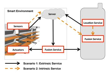
Figure 3. Architecture including information flows for extrinsic and intrinsic scenarios
