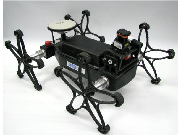
Figure 1: The Asguard v3 platform developed at DFKI. It has mechanical properties similar to those of the Asguard v2 and includes additional sensors. The sensor suite includes a laser range finder, stereo camera, inertial measurement unit and a differential GPS for verification
