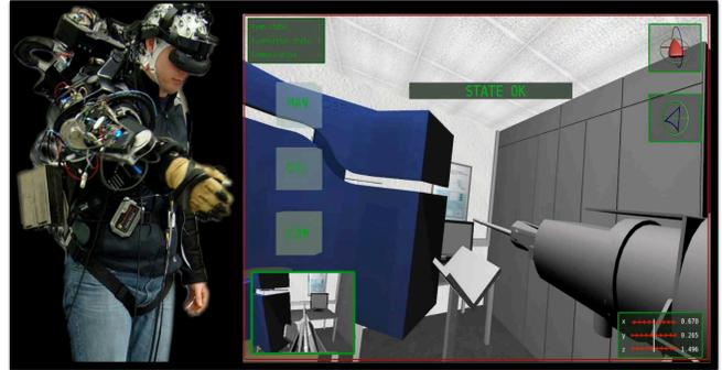
Fig. 1. Experimental setup. Left – operator equipped with exoskeleton, HMD and EEG cap. Right – operator’s view.
