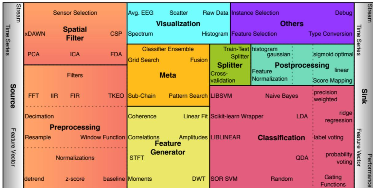
Modularity concept of node chain based on Modular toolkit for Data Processing (MDP)!
