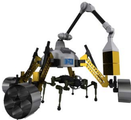
(a) RIMRES systems as CAD models. The six-legged scout CREX is beneath the wheeled rover Sherpa. Attached to Sherpa’s manipulator are two payload-items that form a surface-deployable payload.
