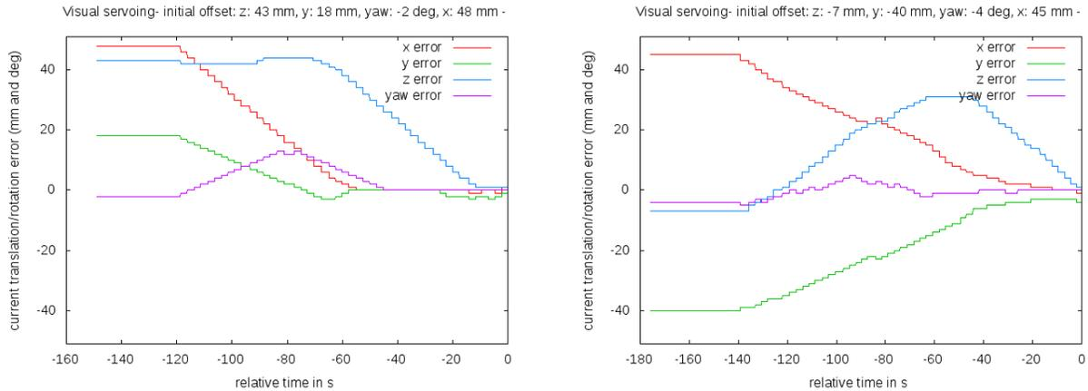
(a) Trend for pose corrections (x, y, z, yaw) for initial offset from taught pose of (48 mm, 18 mm, 43 mm,  $-2^\circ$ ) (b) Trend for pose corrections (x, y, z, yaw) for initial offset from taught pose of (45 mm, -40 mm, -7 mm,  $-4^\circ$ )
