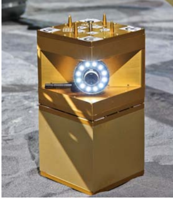
(a) Active payload composed of battery payload-item and camera payload-item. This stack simulates a data generating scientific payload in the RIMRES context.
