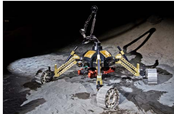
(b) Photograph of final integration status of RIMRES mobile systems. Wheeled Rover Sherpa with manipulator arm and docked six-legged scout robot CREX.
