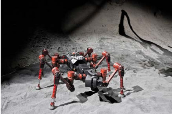
(a) CREX robot in artificial crater environment. CREX is equipped with an electro-mechanical interface for attaching to Sherpa and for carrying payload-items.
