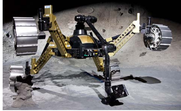
(b) Sherpa using its manipulator as fifth limb. The manipulator is strong enough to bear the weight of the robot, when two legs are lifted off the ground.
