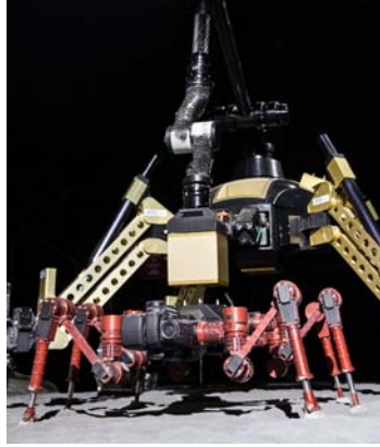
(b) CREX is being equipped with a battery payload-item for extending its range of operation. The payload-item is handled with Sherpa's manipulator.
