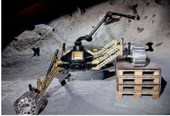
(a) Sherpa using its active suspension to step onto an obstacle. The arm was used to support the robot while lifting each of the front legs.
