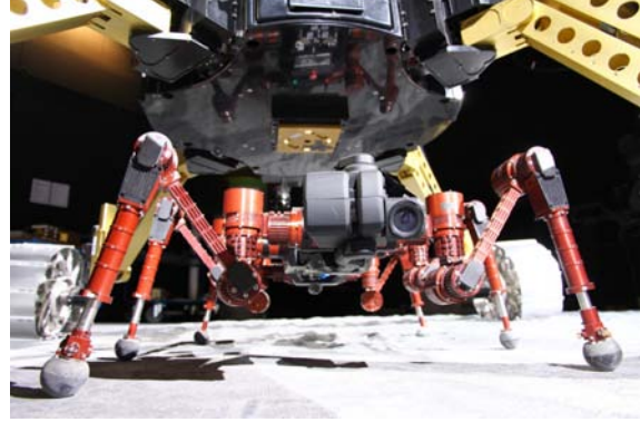
(b) CREX beneath Sherpa after release from Sherpa's electro-mechanical interface (yellow square in the center of Sherpa's belly)
