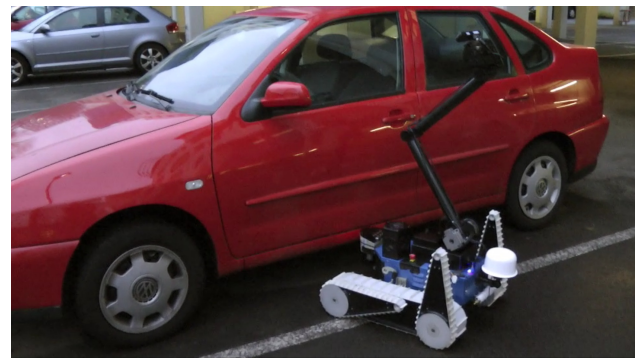
Figure 6. The NIFTi robot looking into a car with the arm. The physical configuration of the arm is written into the ontology for use during reasoning.
