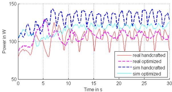
Fig. 6. Power consumption while walking
