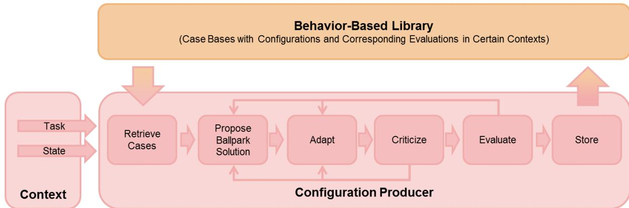
Fig. 5. Processing steps of the case-based reasoning system
