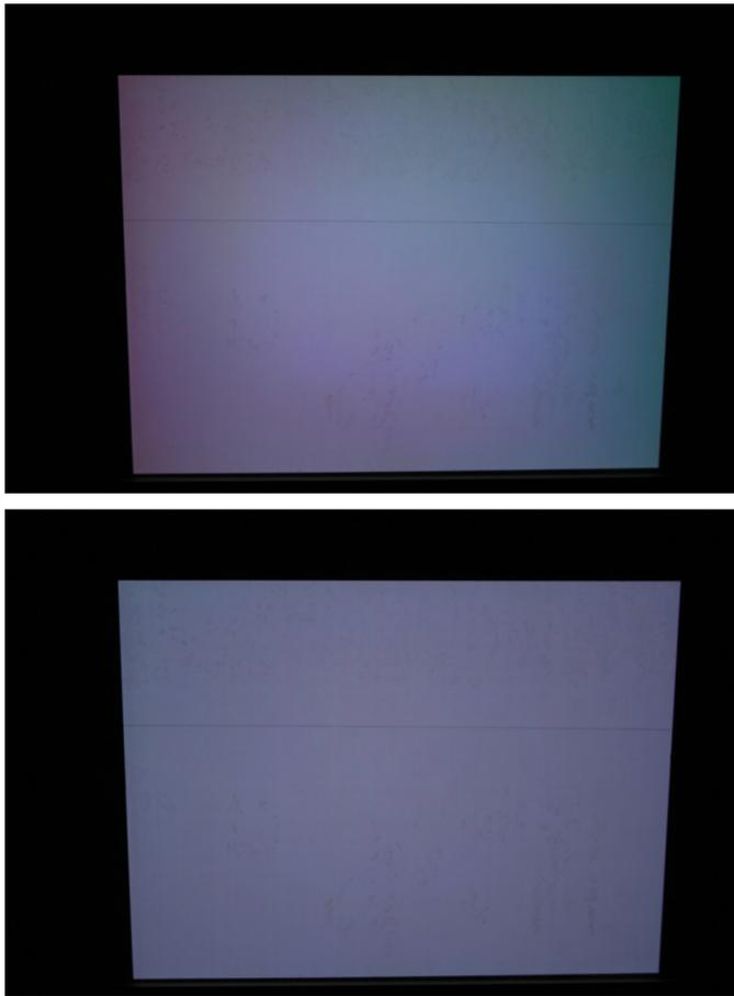
**FIGURE 5** — A projector before (top) and after (bottom) intra-projector correction.
