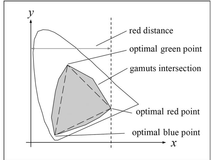
FIGURE 6 — Optimal chromaticity points in the gamut intersection. The red distance to maximize is given as an example.
