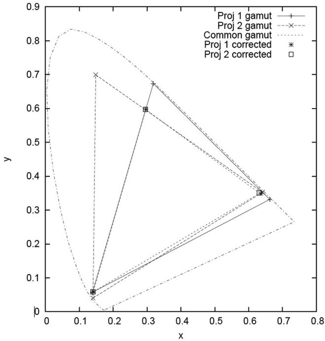
FIGURE 10 — Common gamut and verification for two test projectors.
