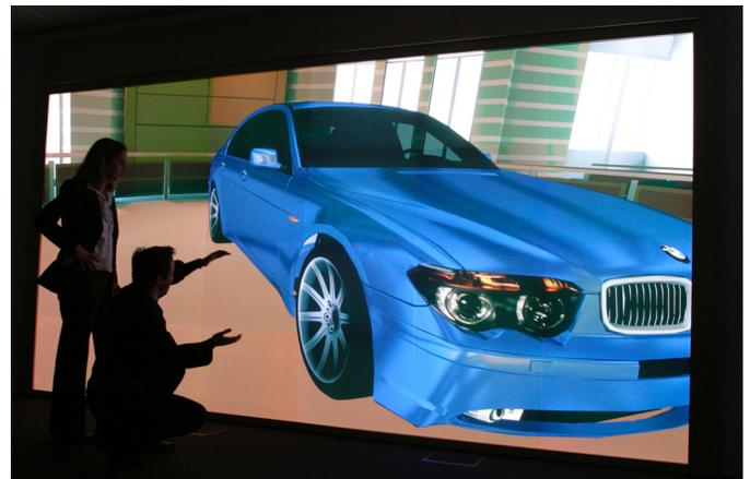
**FIGURE 1** — High-resolution stereoscopic tiled display with 48 projectors (courtesy of Fraunhofer IGD).
