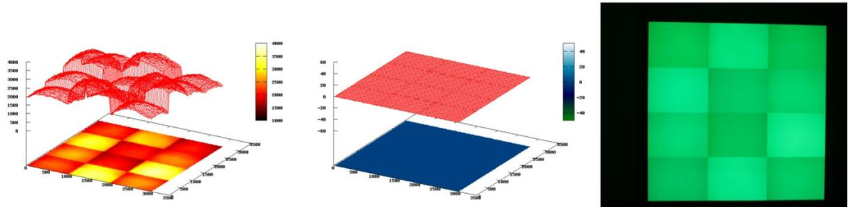
**FIGURE 7** — Intensity profile, absolute correction, and corresponding picture of 12 projectors showing a level of green color before the iterative shading correction.
