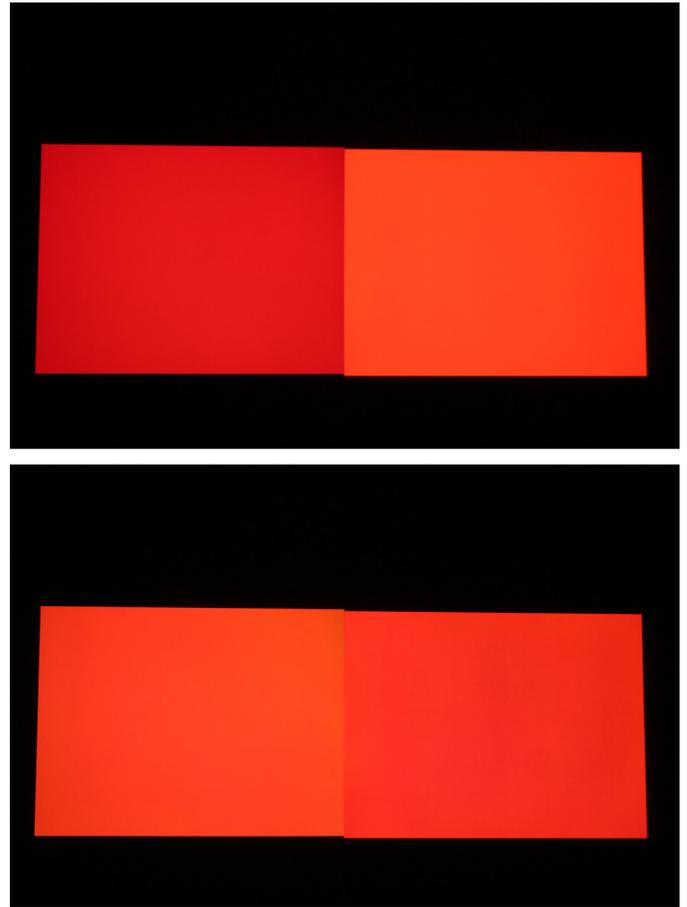
**FIGURE 9** — Two projectors before (top) and after (bottom) correction.
