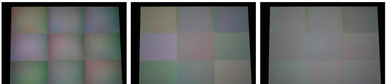
FIGURE 12 — A subpart of the wall with nine projectors before any calibration (left), after intra-projector calibration (middle), and after inter-projector calibration (right).
