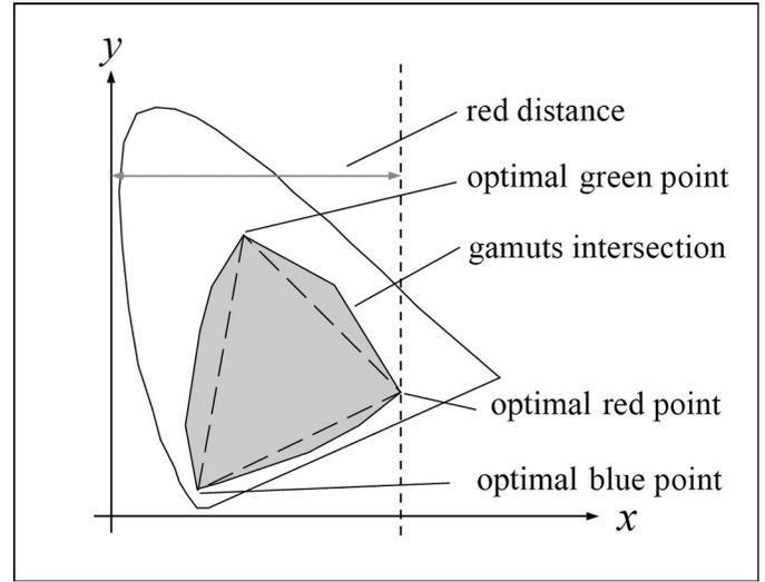
FIGURE 6 — Optimal chromaticity points in the gamut intersection. The red distance to maximize is given as an example.
