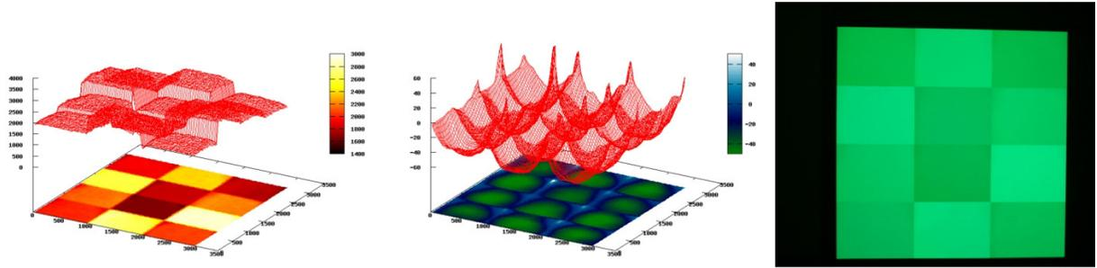
**FIGURE 8** — Intensity profile, absolute correction, and corresponding picture of 12 projectors showing a level of green color after the iterative shading correction.
