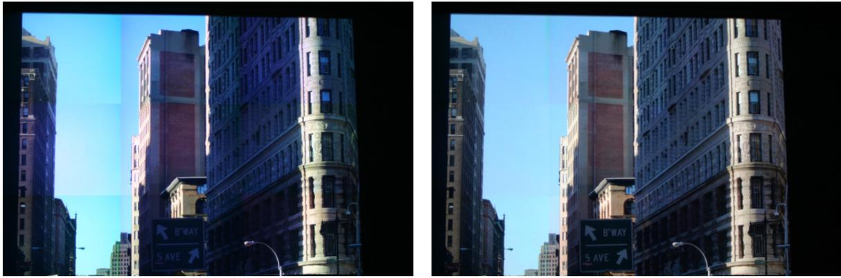
FIGURE 13 — Example of corrected image: before correction (left), after intra-projector and inter-projector calibration (right).
