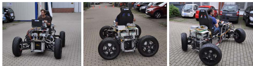
Fig. 3. Ackermann, sideways and turn-on-the-spot drive modes
