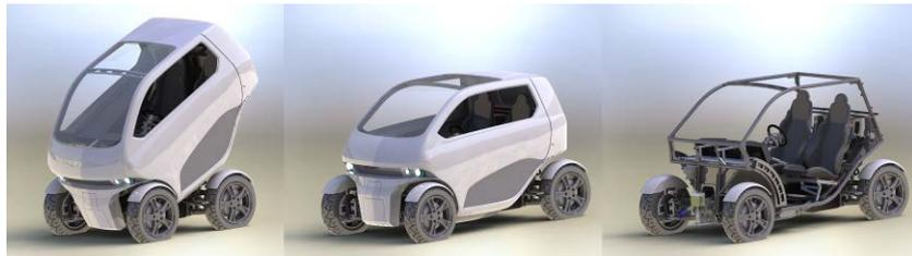
**Figure 1: Folding EOsc2 for reduced parking space and higher maneuverability**
