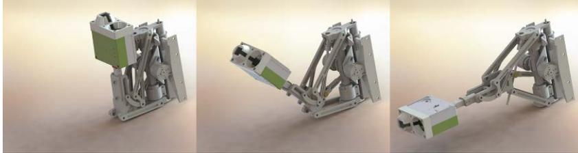
Figure 3: EOsc2 Docking Interface in different folding positions
