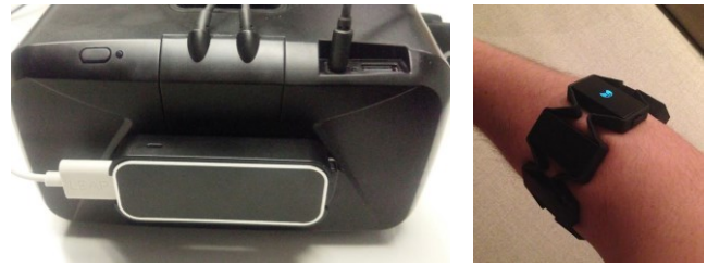
Figure 2. Oculus Rift with attached LEAP Motion for hand interactions such as button presses (left) and the arm-worn Myo to facilitate walking via natural arm movements (right).
