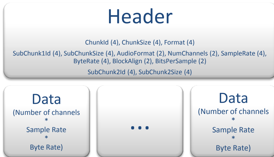
Figure 2.8: WAVE format overview. Each segment of the both Header and Data chunks is presented with its size in braces
