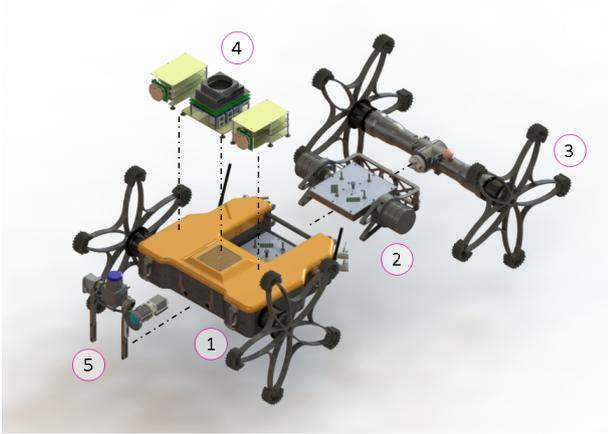
Figure 5. Exploded view of Coyote III showing its main sub-assemblies
