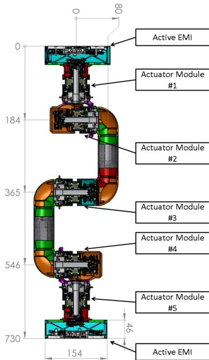
Figure 8. Proposed modular 5 DoF manipulator for PLI handling
