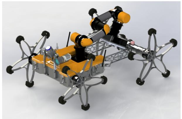
Figure 1. CAD model of Coyote III equipped with its manipulation device
