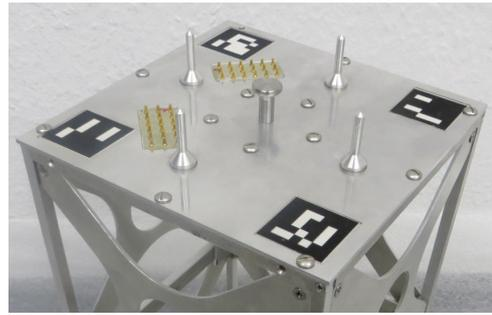
Figure 7. Passive EMI attached to PLI core structure (PLI baseline dimensions:  $154 \times 154 \times 150$  mm)
