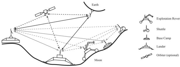
Figure 2. Schematic drawing of the implementation of a logistics chain using a heterogeneous team of mobile and stationary robots (arrows represent possible communication links)
