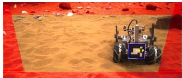
Figure 9- Scout Localization in the camera field of view
