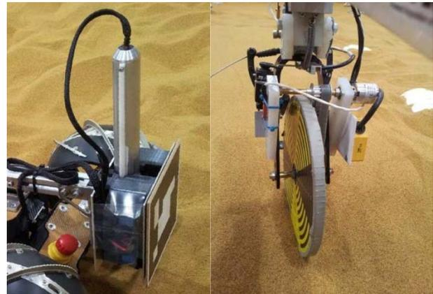
Figure 5- mDCP attached to the scout (left) and WB in front of the primary (right)
