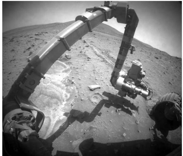
*Figure 1 NASA's Spirit on sol 2052 in loose soil (white sand on the left) after the wheel broke through the darker crusty surface layer (Photo credits: NASA/JPL-Caltech)*
