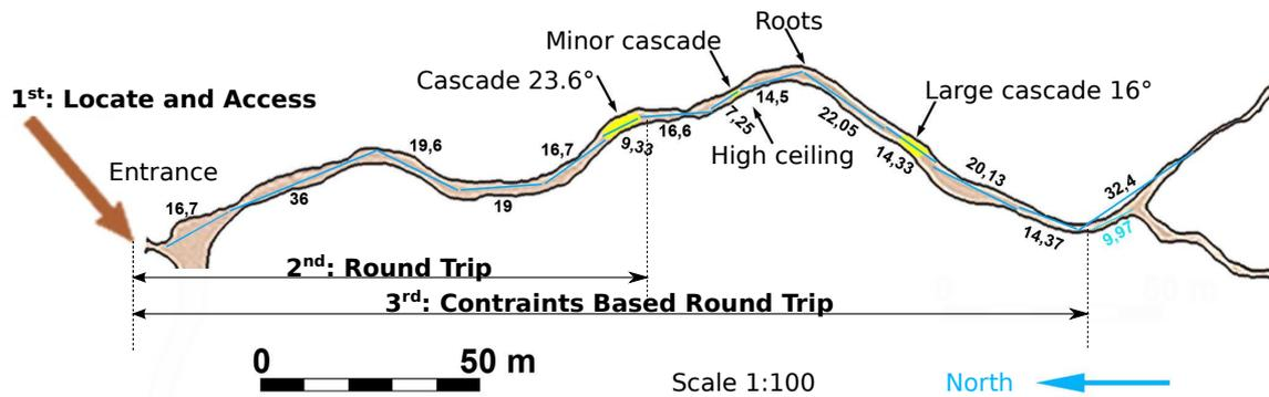
Figure 6. Traversal view of the lava tube in which the system will perform exploration and 3D mapping in three phases: Find and Access (1), Position Based Exploration (2) and Constraints Based Exploration (3). The numbers are distances (in meters) taken with a measuring tape inside the cave. Original map Courtesy of Organismo Autónomo de Museos y Centros de Tenerife, map: Sergio Socorro
