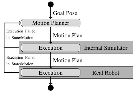
Figure 3. The Closed Loop approach integrates validation from simulation (through the Internal Simulator) and from real execution (through supervision).
