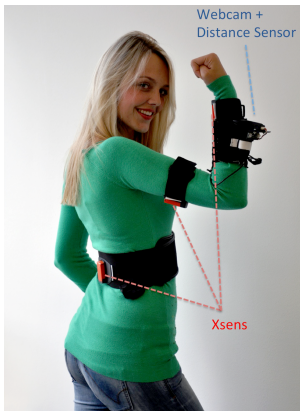
Figure 2. Body-worn sensors: Lower arm mounted camera and distance sensor, Xsens acceleration sensors on forearm, upper arm and back.
