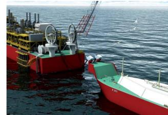
*Tandem offloading: Technip*
