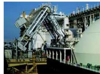
*Side-by-side offloading: FMC*
