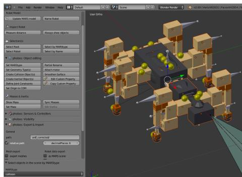
Blender's user interface with the Phobos plugin running. Phobos' custom toolbars are shown alongside the SpaceClimber robot.
