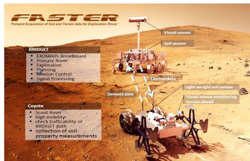
Scenario incorporates autonomous collaboration between a primary rover and a small and agile scout rover used for soil and terrain sensing ahead of a main rover
