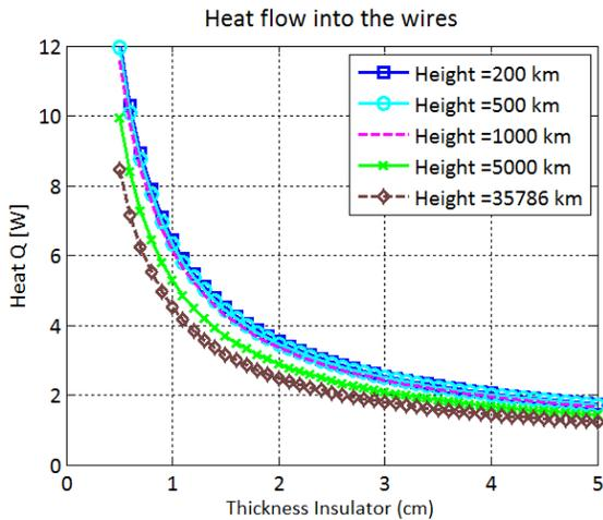
Fig. 6: Convective heat flow to the HTS wires at different altitudes.
