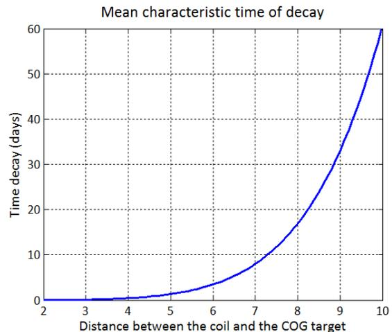
Fig. 9: Mean characteristic time of decay of the angular velocity of the target.
