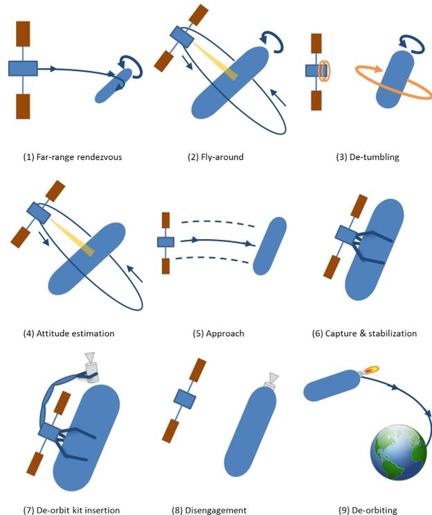
Fig. 1: Schematic illustration of primary mission phases for Agora.
