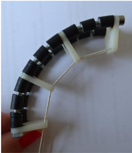
Fig. 10: Prototype of the finger of the clamping device<sup>13</sup>
