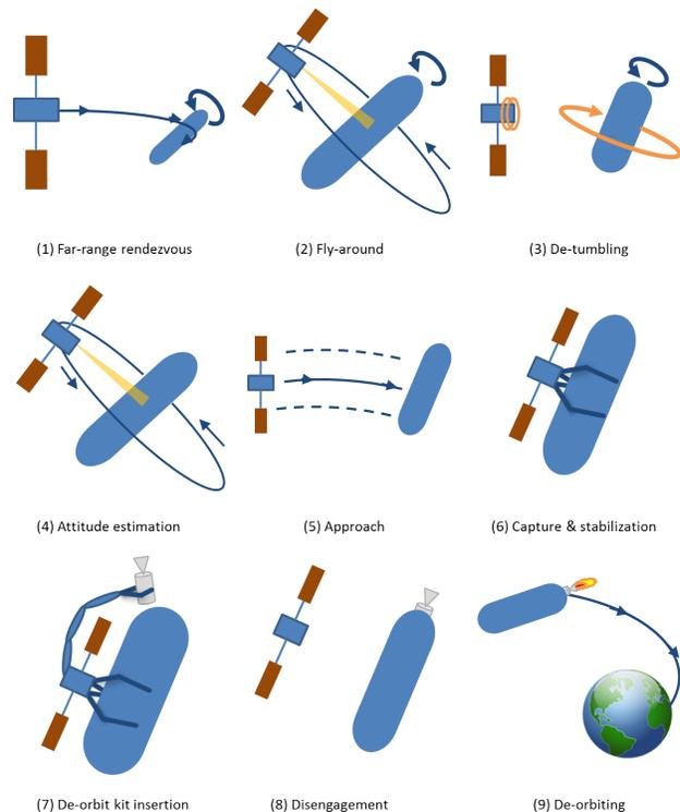
Fig. 1: Schematic illustration of primary mission phases for Agora.
