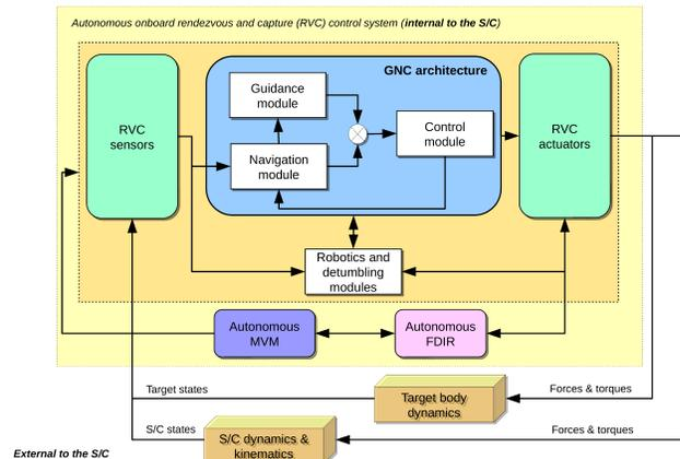
Fig. 8: Autonomous onboard rendezvous and capture control system architecture.<sup>13</sup>
