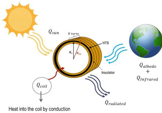
Fig. 5: Heat exchange between the coil and the environment.
