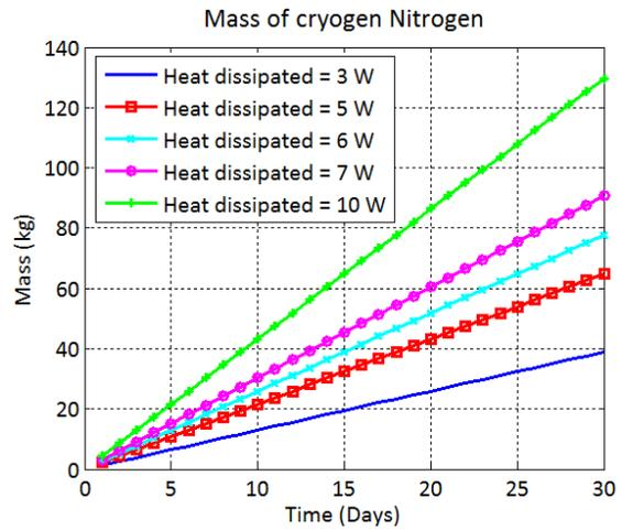
Fig. 7: Mass of nitrogen needed for a dewar-based system for different heat loads and times of operation.
