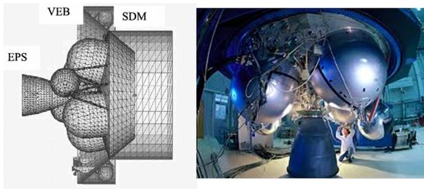
Fig. 4: Ariane-5 upper stage EPS<sup>23</sup> (right photograph from Airbus Defence and Space).
