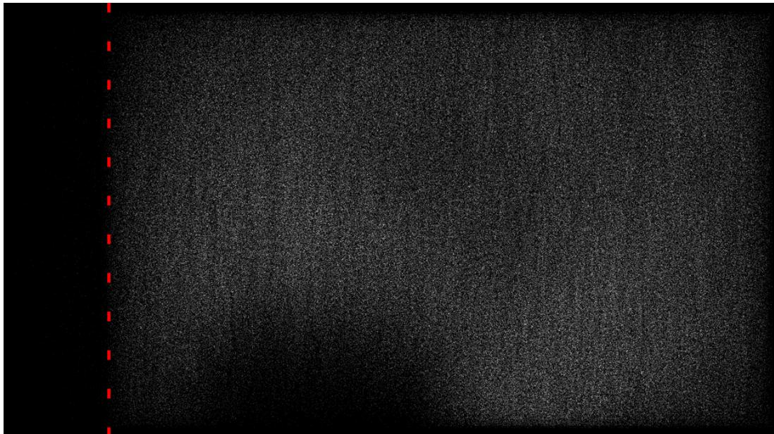
**Figure 4.9:** The location of all detected and stereo-matched features on all left images of the Rostock test sequence (approx 4.500 images) plotted as greyscale image. Dashed red line shows the cropping limit (130 pixels).
