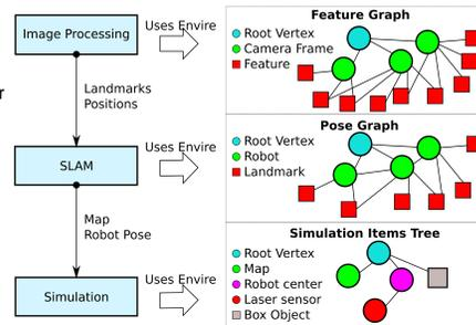
Envire used by three Rock components (left side). Each one adapts the representation to its needs. The different components share information through Rock ports.
