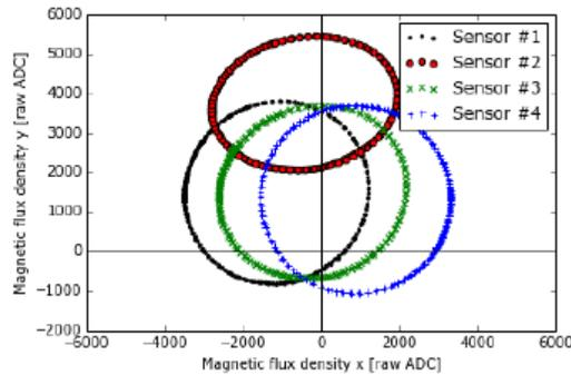
$$\begin{pmatrix} \hat{x} \\ \hat{y} \\ \hat{z} \end{pmatrix} = M_{align} \cdot \begin{pmatrix} sc_x & 0 & 0 \\ 0 & sc_y & 0 \\ 0 & 0 & sc_z \end{pmatrix} \cdot M_{si} \cdot \begin{pmatrix} x \\ y \\ z \end{pmatrix} - b_{hi}$$
