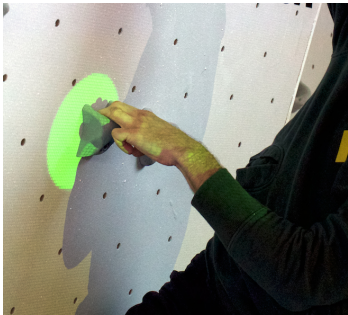
Figure 5: Using perspective projection and blob detection, the selected hold is highlighted.
