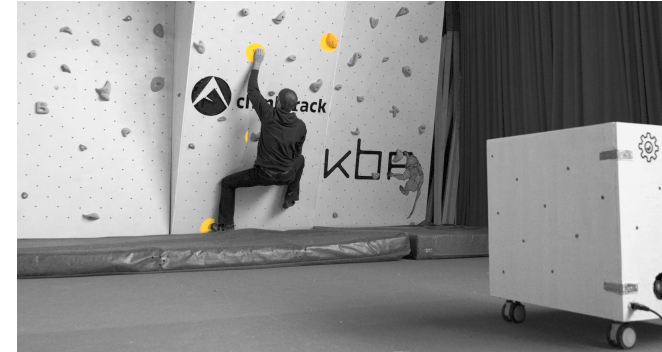
Figure 4: Setup of the system. The betaCube can be placed in front of an arbitrary climbing wall. Holds are highlighted by a projector.
