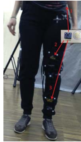
Figure 7: Real test setup. The red arrows show three IMUs which are mounted on pelvis (1, not visible), upper leg (2) and lower leg (3).
