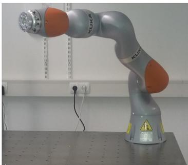
**Figure 1:** KUKA iiwa R820 lightweight robotic arm used for the experiments
