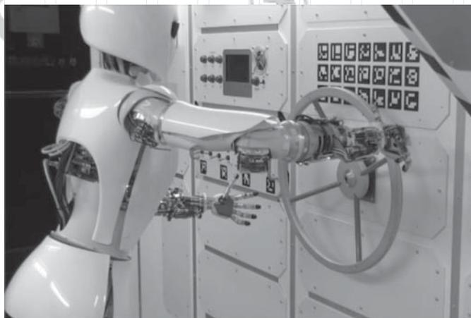
Figure 5.29 Robot AILA using whole-body control to perform some tasks within a mock-up International Space Station. (Courtesy DFKI GmbH.)
