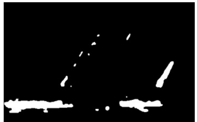
Fig. 6: Effect of morphological opening on the image.
