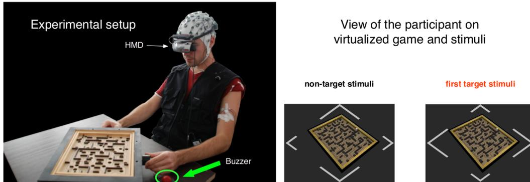
Figure 5: Experimental setup and view of the participants through the head mounted display (HMD) on the virtualized game and presented infrequent first target and frequent non-target stimuli.
