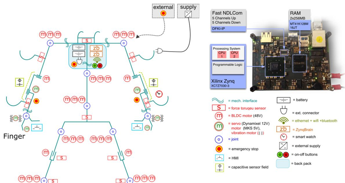
Figure 2: Left: Plan of electro-mechanical components within the exoskeleton robot. Right: The ZynqBrain processing platform used as central processing unit.
