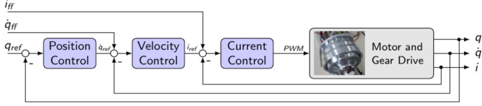
Figure 3: Low-level control architecture for actuators.  $q$  is the angular position,  $\dot{q}$  is the angular velocity and  $i$  is the motor current.
