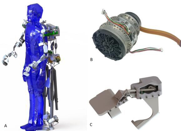
Figure 1: A: full-body exoskeleton. B: series elastic actuator used at the elbow. C: active hand interface support grasping tasks and hand opening.
