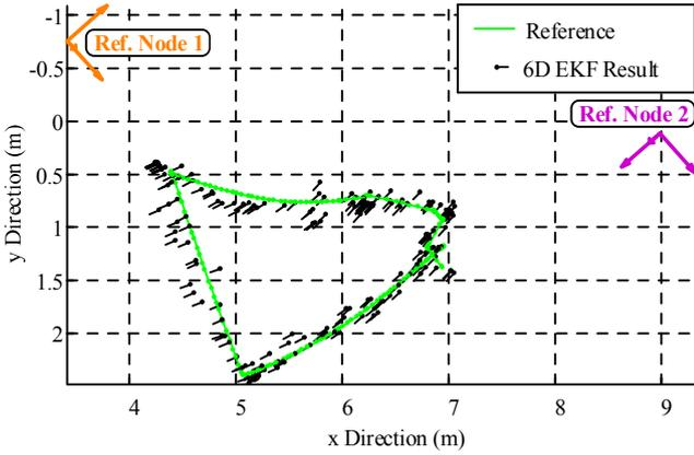
Fig. 5. Measured trajectory in DFKI space exploration hall (top view).
