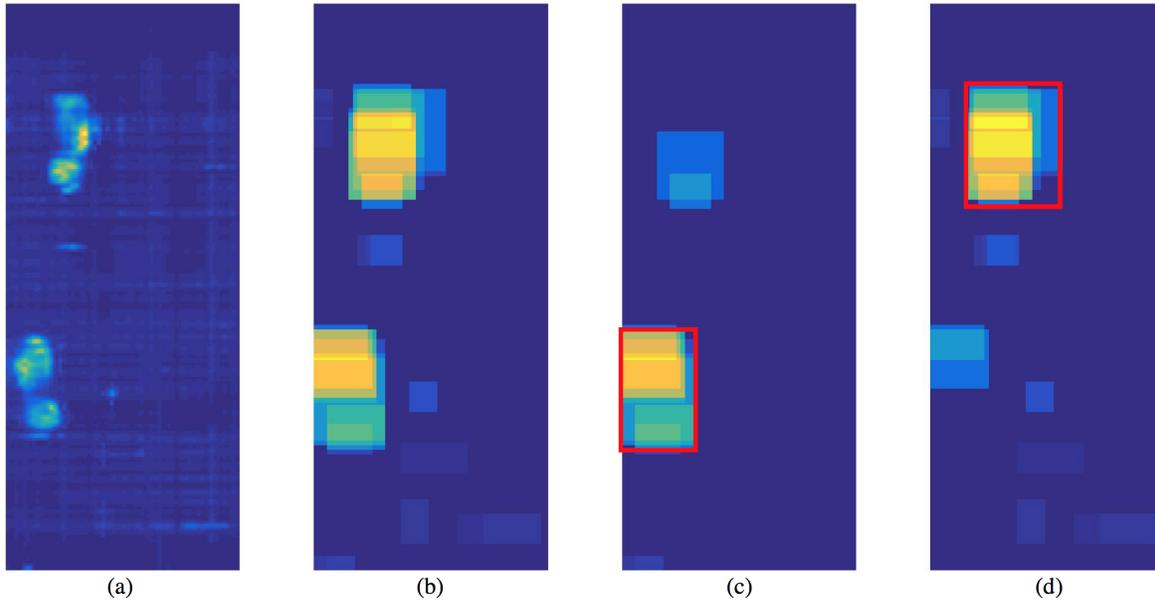
Fig. 4. Step segmentation: (a) sum of pressure mapping over a walking event, (b) all bounding boxes during the event, (c) detection of the first step, (d) detection of the second step
