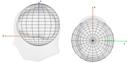
Fig. 1. Spherical Head Model – The x-axis points to the right, the y-axis to the front, and the z-axis runs through the vertex.
