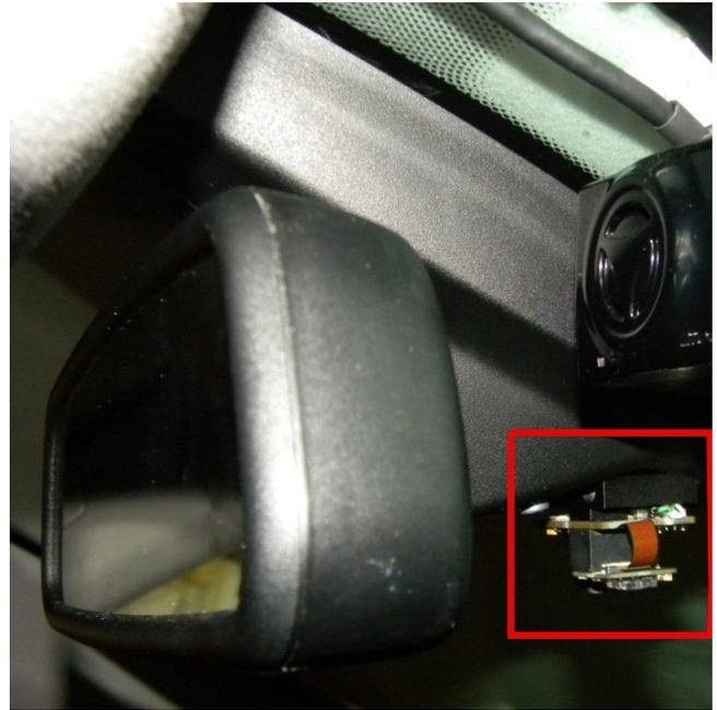
Figure 2: The camera (shown in red box) in the car.
