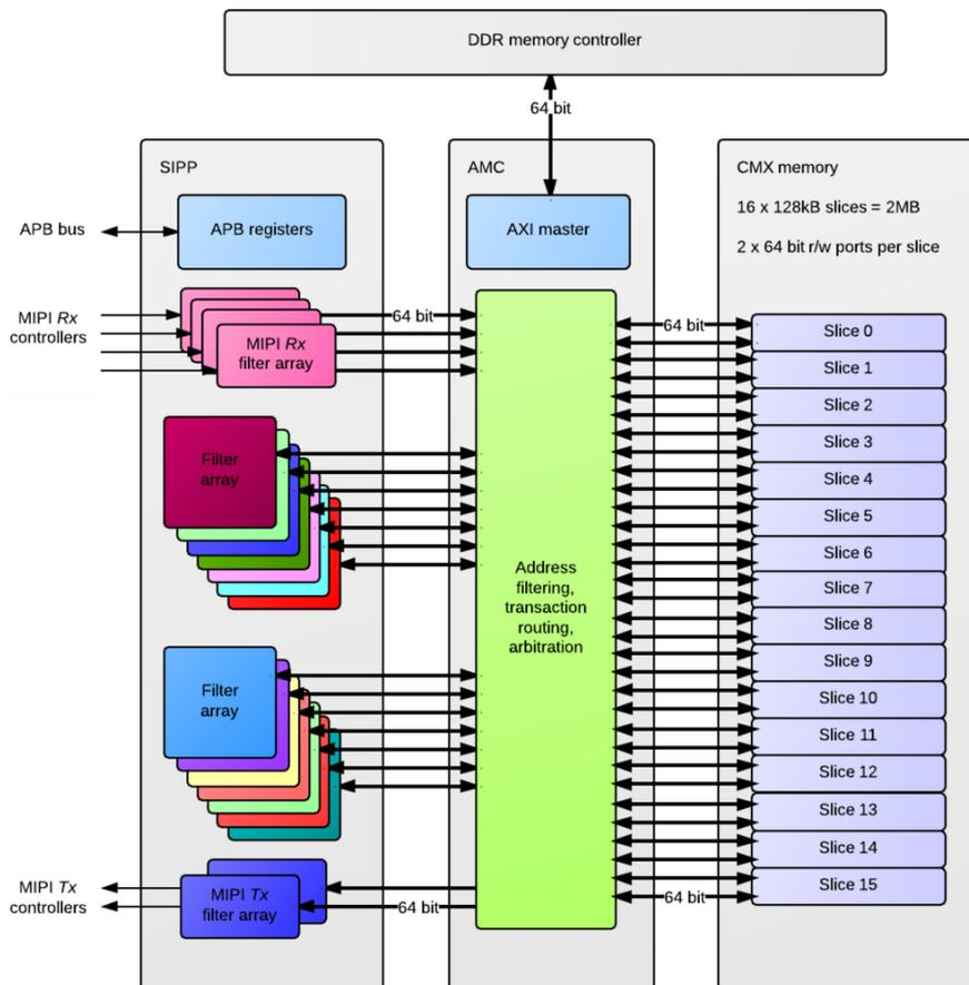
Figure 7. Block diagram of SIPP accelerator, AMC and connections to CMX .
