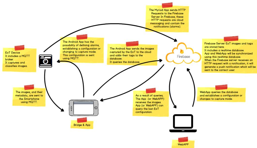
**Figure 21.** Architecture of the versatile mobile camera demonstrator.
