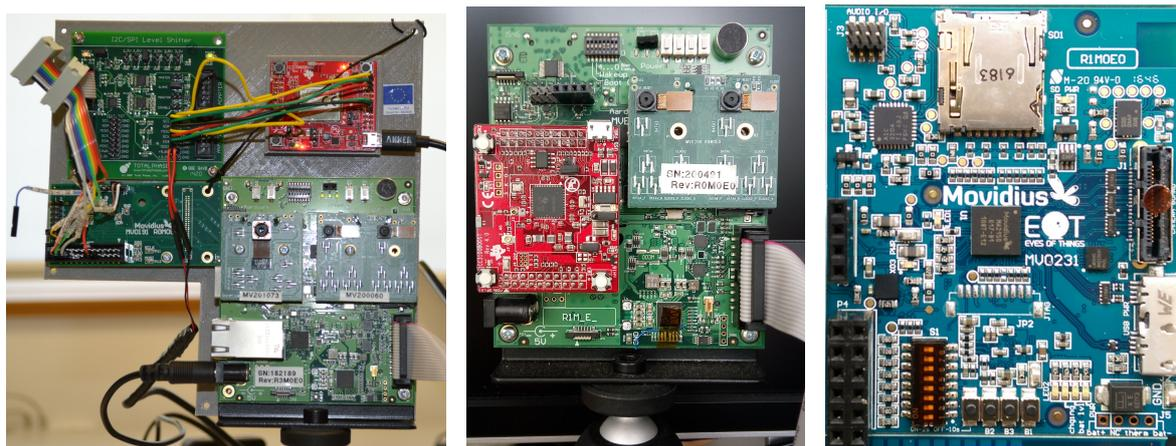
**Figure 1.** Development of Ears of Things (EoT) boards. Sizes, from left to right (in mm): 200 × 180, 100 × 100, 57 × 46.
