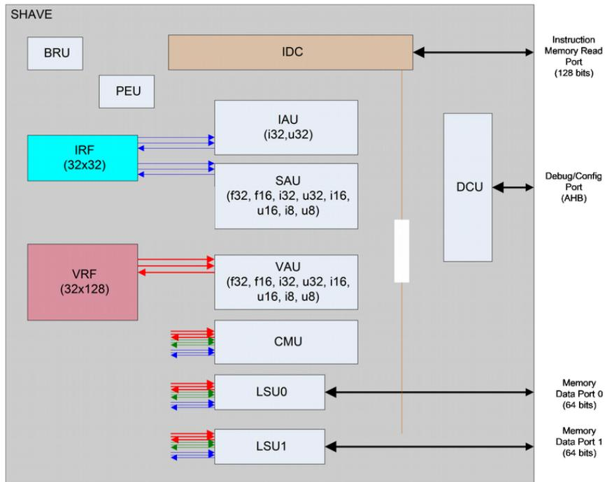
Figure 6. SHAVE internal architecture.
