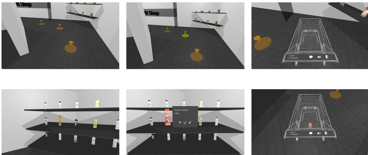
Fig. 7. **Head Pointing.** Here, the user looks at a nearby waypoint in order to be moved. Then, a product is placed into the shopping cart after it has been selected. Finally, the total sum and amount of items is displayed on the shopping cart's handle.
