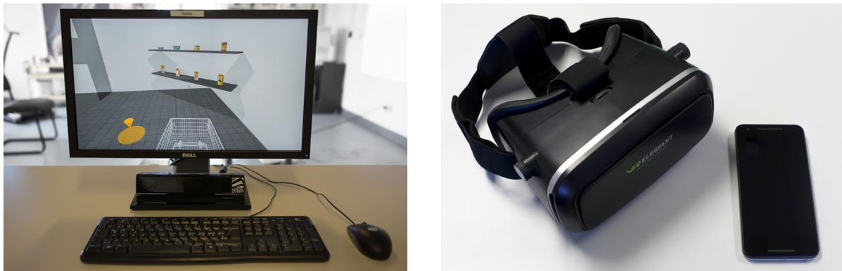
Fig. 9. This figures show the **output devices** we used for our prototype. On the left: 22 inch display with Microsoft Kinect 2 for speech input and a standard mouse for camera control. On the right: a common smart-phone VR case and LG Nexus 5X.
