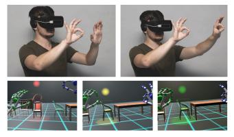
Figure 1: Bi-manual mid-air interaction in Virtual Reality.
