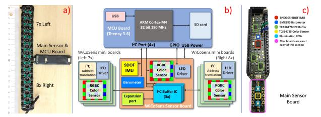
Figure 1. a) WiCoSens - A wrist worn color sensing device with magnetic locking. b) WiCoSens system architecture. c) Main sensor board (top view).
