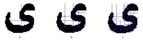
Figure 7. The hierarchical geometric centroids for " $\mathcal{G}$ " character a) in the first level b) in the second level c) in the third level
