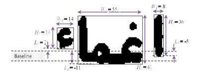
Figure 5. Three features of sub-words of a word include height(H), width(W) and the vertical distance (L)
