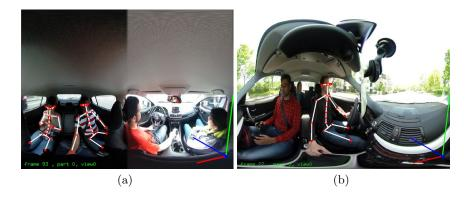
Fig. 2. 3D pose tracking of passengers with the 3D skeleton superimposed for (a) passengers and (b) driver
