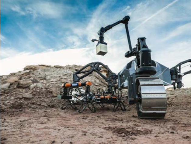
Figure 7. PLI handling between Coyote III and the end-effector of SherpaTT
