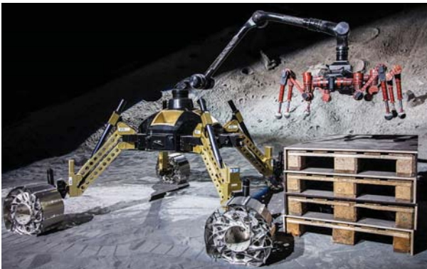
Figure 8. End-effector of Sherpa carries CREX
