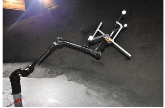
Figure 12. Setup on the end-effector for the repeatability test
