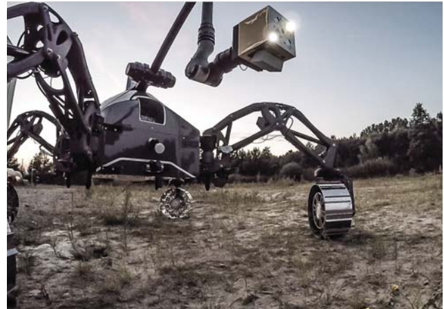
Figure 6. Extending of work ability by using of the sampling module docked on the end-effector
