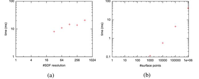
Fig. 3: Scaling behaviour of QUALIFY(A, B) with respect to (3a) varying SDF resolutions, and (3b) point-based boundary representations of increasing sizes for Armadillos configuration.
