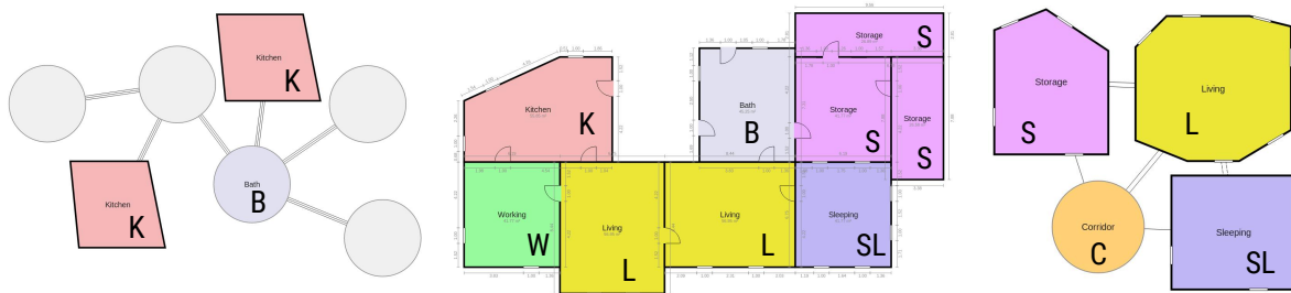
Figure 7: Examples of evaluation queries. Bubbles denote rooms without specific functionality and/or geometry. C denotes the CORRIDOR room type, others are WORKING, LIVING, STORAGE, SLEEPING, BATH, PARKING, and KITCHEN.
