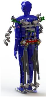
Fig. 18: ACTIVE ANKLE applied as 3-DOF hip and ankle joints in the RECUPERA full body exoskeleton.
