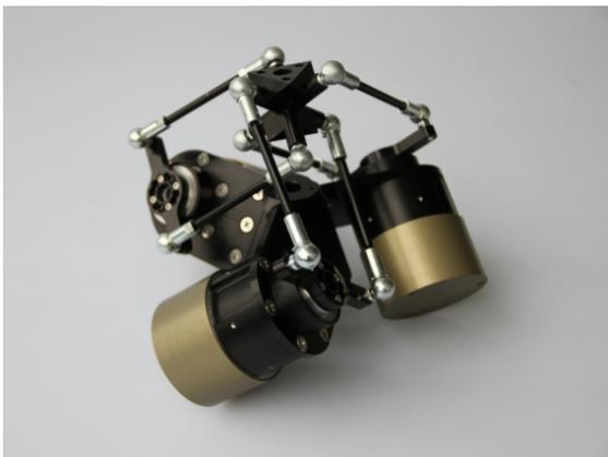
Fig. 1: A built-up prototype of the 3-DOF ACTIVE ANKLE incorporating actuators and control electronics. Its technical specifications are outlined in Section 2.2.
