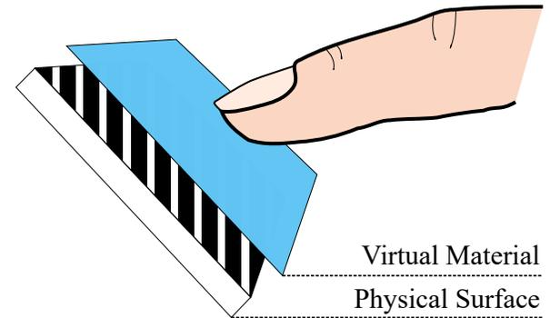
**Figure 1:** The concept of augmenting texture perception by overlaying a physical structure with a virtual texture, where the physical structure is created by a 3D printer.
