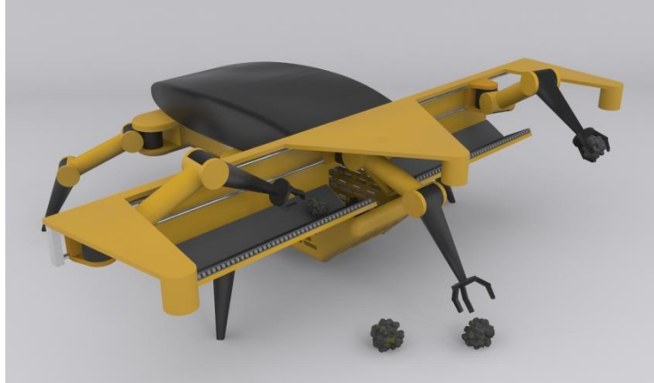
Figure 13 Illustrative drawing for robotic platform with minimal-invasive ground contact and individual handling of manganese nodules
