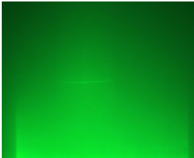
Figure 5 Camera image at 1.8m distance to pipe and 5.1 FTU[2]
