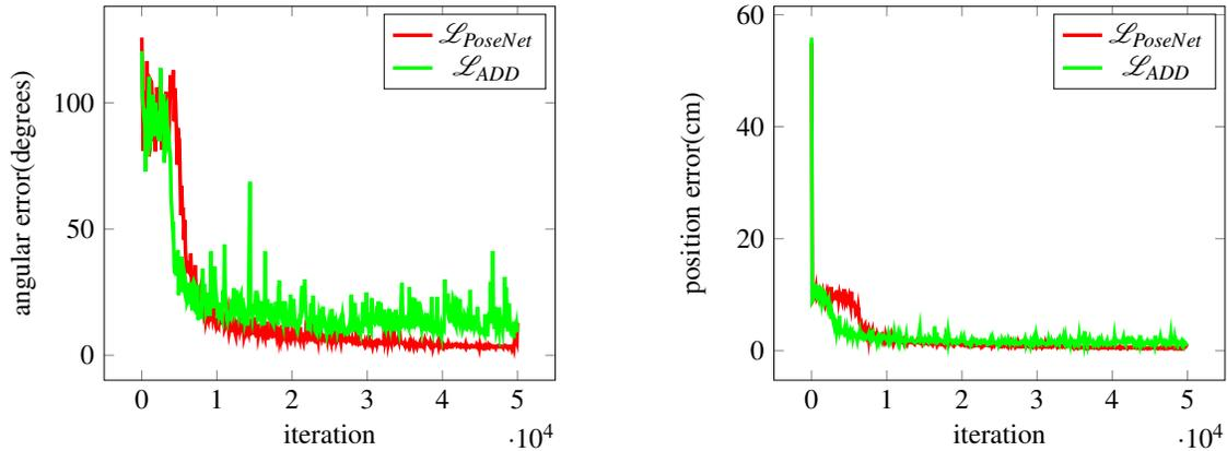
Figure 4: Comparison of network training with the two proposed loss functions  $\mathcal{L}_{PoseNet}$ ,  $\mathcal{L}_{ADD}$
