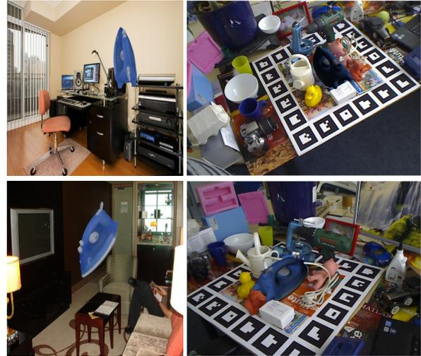
Figure 1: We use only synthetic images to train a CNN to regress the 6DoF pose of objects in real images
