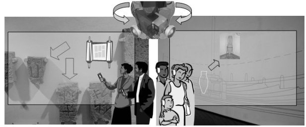
Figure 1: A steerable projector is used to display group relevant information on or nearby exhibits. Personal devices (such as a PDA or a personal audio device) provide individual annotations.
