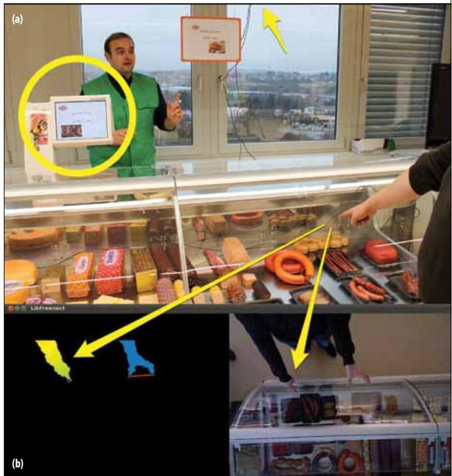
**Figure 2.** Interactive fresh food counter: (a) system setup with scale (indicated by the circle) and Microsoft Kinect camera installed 2.5 m above the counter (indicated by the upward-pointing arrow); (b) the scene as captured by the RGB camera (right) and the depth view (left).
